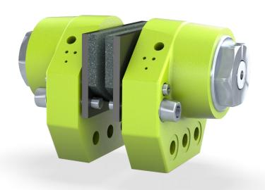
The disc spring pack must be adjusted to compensate for brake lining wear and to maintain full brake capacity. An extension of the brake piston through the adjustment nut gives an easy visual way to tell when adjustment is needed.
