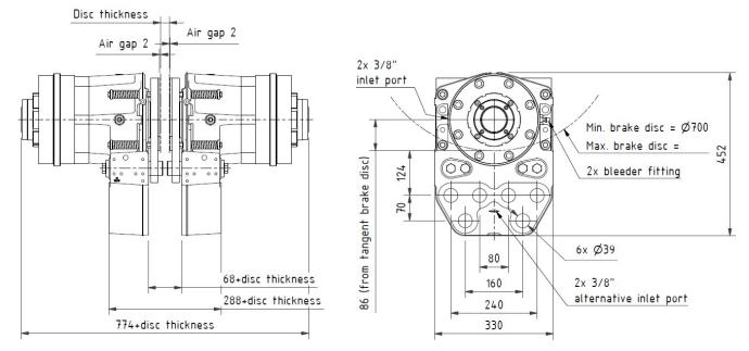
Maximum Shaft flange diameter = Brake Disc diameter øD - 440 mm
