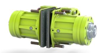
The SKP 180S allows a brake pad lining wear of up to 3 mm before replacement is required, which could be a lifetime's use in applications where the brakes are purely used statically and/or in emergency situations. The brake piston extends through the rear lock nut to give an easy, visual way to tell when replacement is needed. The SKP 180 series also includes the SKP 180A, where disc spring packs can be adjusted to compensate for lining wear.
